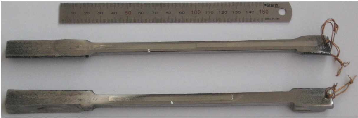
Fig. 3. Test specimens with fatigue gauges
